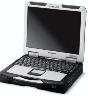
Panasonic Toughbook: CF-31 Fully ruggedized computer. Designed using MIL-STD-810f test procedures. Full magnesium alloy case, vibration and drop-shock resistant, built in carry handle, removable shock mounted hard drive, moisture and dust resistant design. 13.3" monitor that is available with touch screen options.
